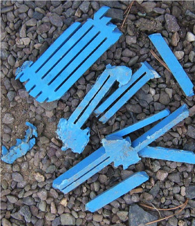
Fragments of screen broken during 'fishing operations'
